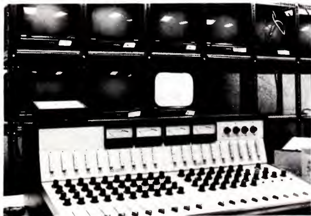
Studio B is major production studio. Control Room includes a new Grass Valley switcher model 1600 and a flexible audio console.
