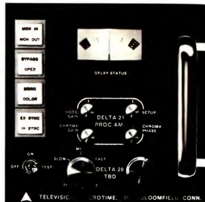
TMI's exclusive built-in Delta 21 proc amp and Delta 28 TBD.
